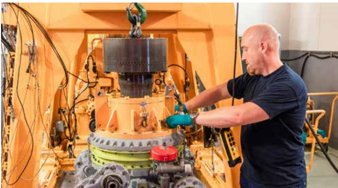
Olav Topland monterer Mk1 Main Gearbox i test benk.
